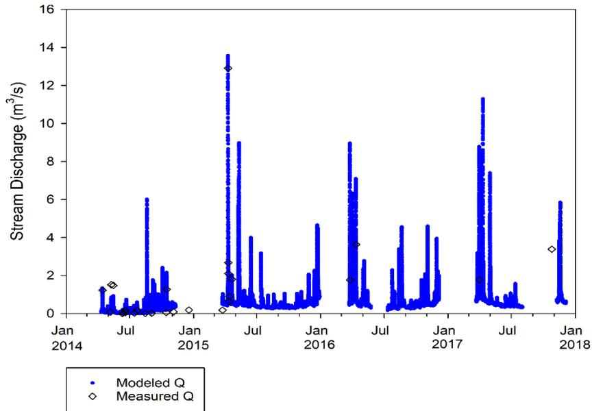
Figure 20. North Upstream site hydrologic modeling.
