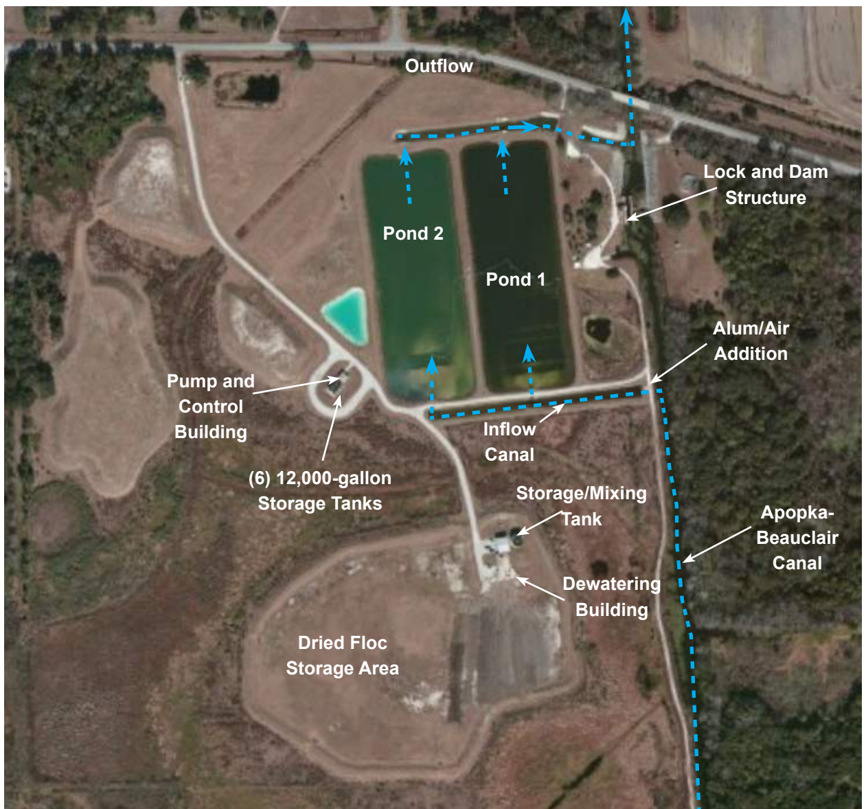
Figure 11. Apopka Beauclair Canal Nutrient Reduction Facility. Modified from Harper (2013). Graphic is for informational purposes only and illustrates some of the infrastructure components that may be included in a large-scale alum injection facility.
